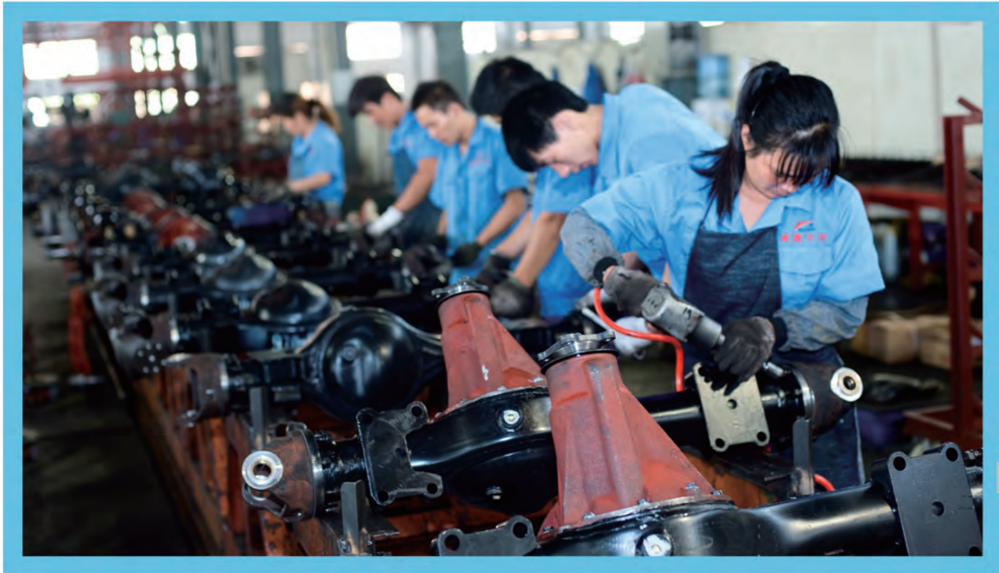
■ 前驱桥装配线 ASSEMBLY LINE FOR STEER & DRIVE AXLE
