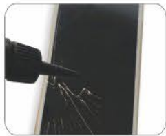
DROP THE RESIN ON THE BREAK AREA
