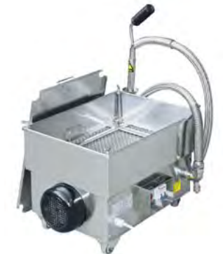
Oil Filter Cart FF-XOFC20 Dimension(LxWxH): 450x330x350 mm Oil Filtering Capacity: 5 Liters/ min Pump Flow: 20 Liters/ min Discharge Pressure: 0.33 Mpa Power: 0.55 Kw, 220-240 V N/W: 4.6 Kgs 1. Rational and technological design, high efficiency of oil fitting 2. Equipped with switch protection cover, safe and unique.
