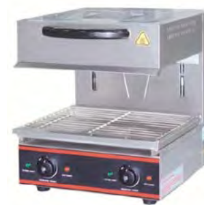
Electric Lift Salamander HK-YES-600 Dimension(LxWxH): 600x450x500 mm Power: 4 Kw, 220-240 V Temperature Range: 50-300 °C Heating Zone: 590x320 mm Up & Down Travel: 0-140 mm N/W: 49 Kgs
