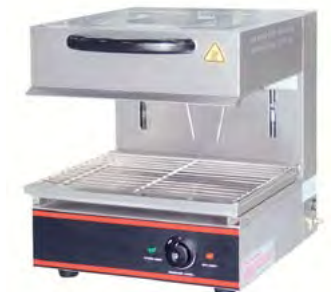
Electric Lift Salamander HK-YES-450 Dimension(LxWxH): 450x450x500 mm Power: 2.8 Kw, 220-240 V Temperature Range: 50-300 °C Heating Zone: 440x320 mm Up & Down Travel: 0-140 mm N/W: 38.5 Kgs
