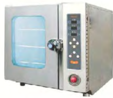
Electric Combi Steamer MC-31.3K2 Dimension(LxWxH):670x710x678 mm Voltage:3~380V/50Hz Power: 6 Kw Max Capacity:3 pcs GN 1/1 N/W:44 Kgs
