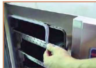
Removable door gasket for easy replacement
