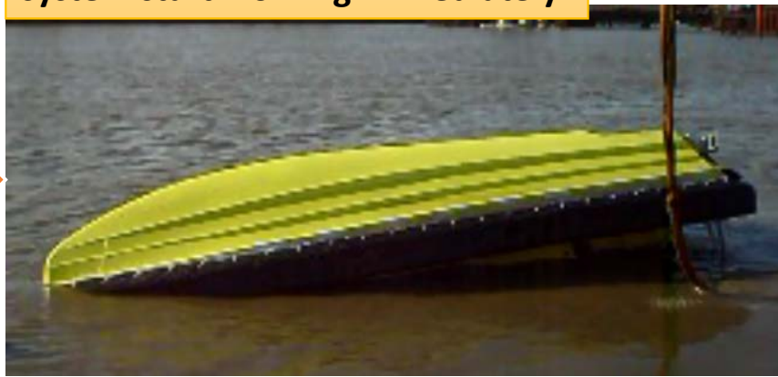
Automatic inflatable self-righting system start working immediately
