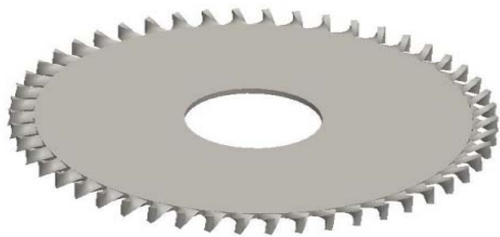
MS007 Earth washer Outdia 30, inner dia 8 Thickness 1.5mm
